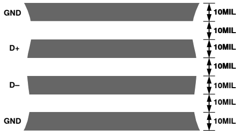
Figure 19. Arrangement of Signal Tracks
