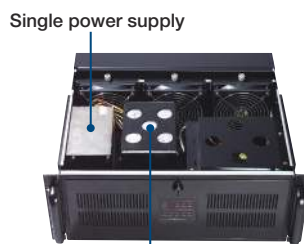
Single power supply Extra drive bay which can hold up to three 3.5" HDDs
