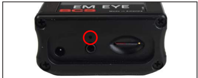
Figure 7. Location of the reset button at the bottom of the EM Eye Meter
