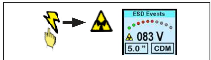
Figure 20. Changing the filter from “True ESD mode” to “All Signal mode”
