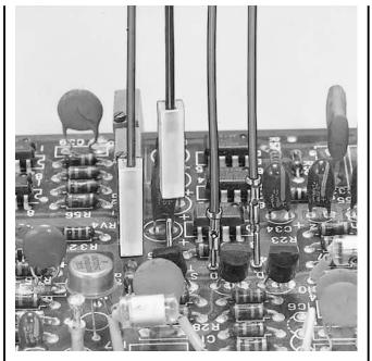
This small single-circuit connector connects to 1.0mm and 1.3mm diameter pins and requires only minimal space for connection of wires to high-density printed circuit boards.
