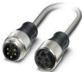
Bus system cable, DeviceNet, 5-position, PUR halogen-free, Gray RAL 7001, Plug straight 7/8"-16UNF, on Socket straight 7/8"-16UNF, Cable length: 10 m
