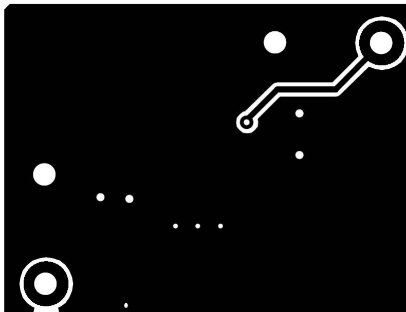
Figure 65. Bottom Layer of Example Converter Layout
