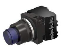
30mm BlackMax, Epoxy Coated Corrosion Resistant Complete Metal Unit PTT / Illuminated Pushbutton Full Voltage, 24V AC/DC LED Lamp Extended Button Plastic Lens, Blue 2 Position Momentary with 1 N.O. - 1 N.C. Heavy Duty Contacts, A600/P600 UL Listed, CSA Certified NEMA 1,3,3R,4,4X,12,13 & Automotive Standards
