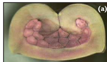
Significant flash can be generated with excessive anvil to crimper clearance, as shown by nominal design condition (a) and +0.003 in over nominal condition (b)
