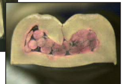
Visible Deformation of Outer Crimp Surface as a result of Indentation from Material Buildup on Crimper
