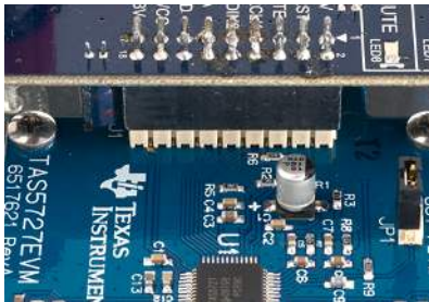
Figure 4. Connecting TAS5727EVM to MC57xxPSIA
