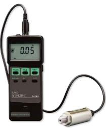
These pressure transducers come with the thread size of 1/4" NPT (per inch 18 teeth) and one adapter connector with the tread size of 1/4 inch PS (per inch 19 teeth). To use the 1/4" NPT threads directly, you will need to remove the adaptor connector from the transducer manually.
