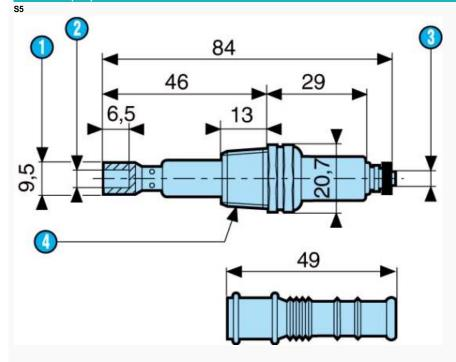
Suitable for high pressures and high temperatures. For use up to 350 °C and 15 kg/cm2 Metal parts of stainless steel, isolated by ceramic. 3/8" BSP mounting thread.
