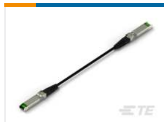
TE Part #2821222-5 SFP28 DIRECT ATTACH CA, 0.5M, 30AWG
