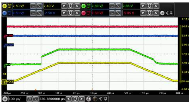
Figure 6-11. V_{OD(DOM)} Over V_{CC}
