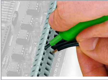
Inserting a conductor via 3.5 mm screwdriver.
