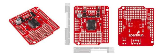
**Description:** The Ardumoto Shield is a dual-motor controller for Arduino. Based on the L298 H-bridge, the SparkFun Ardumoto can drive two DC motors up to 2A per channel. Combined with an Arduino, the Ardumoto makes a fantastic controller platform for RC vehicles or even small autonomous robots. It's now easier to use, featuring control signal LEDs, while also being much more flexible for advanced users.
