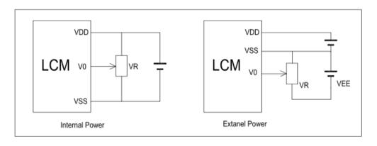
VDD-V0: LCD Driving Voltage
