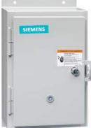
Non-reversing motor starter, Size 0, Three phase full voltage, Solid-state overload relay, OLRelay amp range 5.5-22a, 110 120/220 240VAC 60HZ coil, Non-combination type, Enclosure type 12, Dust/drip proof for indoors, Extra-wide enclosure
