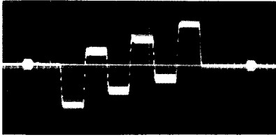
Fig. 24(c) - CA3072 terminal No. 13, 4.8 v_{p-p} B-Y output, one horizontal line
