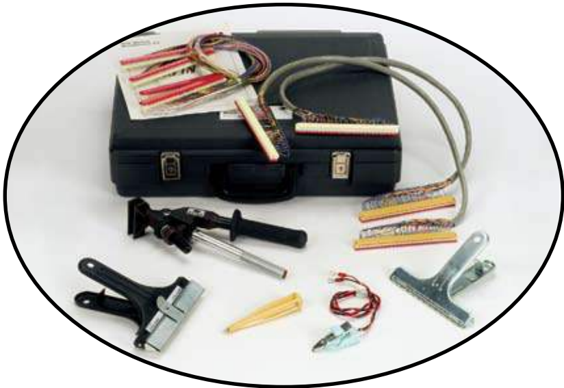
The 3M™ MS™ Module Maintenance Kit 4026-A contains the tools necessary for re-entry of super-mini and super-mate modules. The kit may be used for splice module combinations of two- through seven-way stackable splices.
