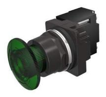
30mm BlackMax, Epoxy Coated Corrosion Resistant Metal Operator, Round Illuminated Twist-to-Release Full Voltage, 24V AC/DC Incandescent Lamp Mushroom Head Cap Small 1.79" (45 mm) Plastic Cap, Green 2 Position Maintained, Twist-to-Release UL Listed, CSA Certified NEMA 1,3,3R,4,4X,12,13 & Automotive Standards
