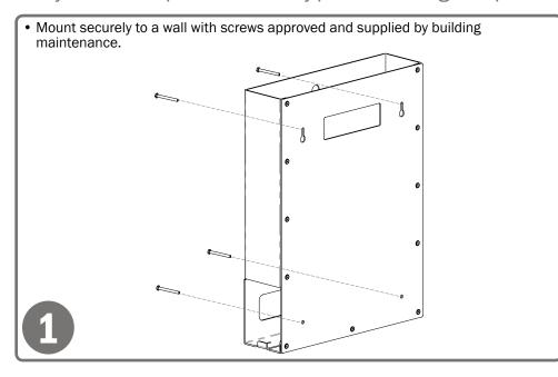
• Dispenser can be mounted onto a BOWMAN® door or wall hanger through the cutout in the back.
