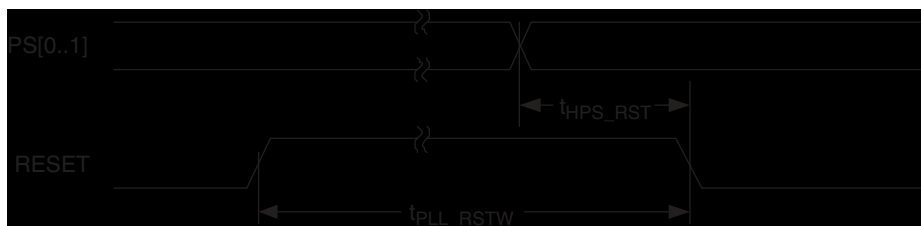
Figure 1-7. RESET and Profile Select Timing
