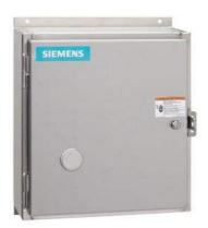
Mechanically held lighting contactor, Contactor amp rating 20Amp 0NC  $\_$  8NO poles, 265-277V 50/60HZ coil, Non-combination type, Encl NEMA type 4X 304 S-steel Water/dust tight noncorrosive
