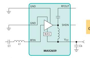
INPUT MATCH L1 = 6.5nH INPUT DC BLOCK C1 = 1800pF SUPPLY BYPASS Cb = 33nF
