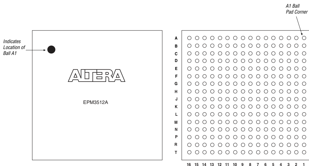
Figure 18. 256-Pin FineLine BGA Package Pin-Out Diagram
