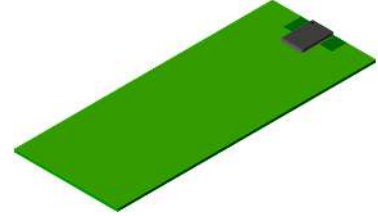
Cell phone config 1 with side ground plane (size: 40 x 100 mm 2 )
