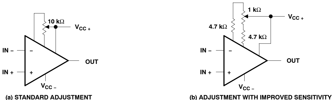
Figure 55. Input Offset Voltage Nulling Circuits
