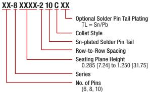
ALL DIMENSIONS: INCHES [MILLIMETERS] ALL TOLERANCES: ±0.005 [0.13] UNLESS OTHERWISE SPECIFIED FOR COLLET CONTACTS ON 0.300 [7.62] CENTERS, SEE DATA SHEET 13008 FOR BIFURCATED CONTACTS, SEE DATA SHEET 13006 CONSULT FACTORY FOR OTHER SIZES AND CONFIGURATIONS
