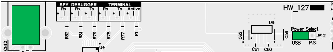
Figure 5.1 : Power Select Jumper Configuration for USB Power
