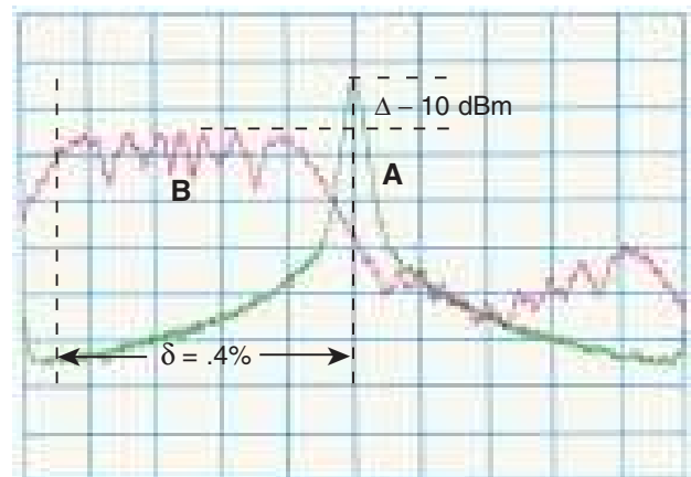
FIGURE 2B. 200MHZ CLOCK OUTPUT IN FREQUENCY DOMAIN (A) SPREAD-SPECTRUM OFF (B) SPREAD-SPECTRUM ON
