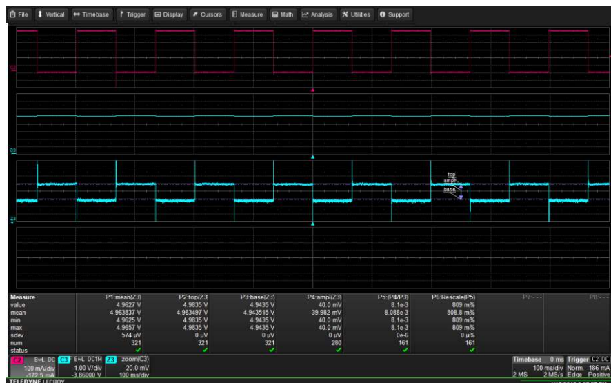
Figure 1: Using parameters and parameter math to measure load regulation
