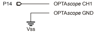
Figure 1-14: High and Low signals circuit schematic
