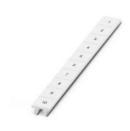
Zack marker strip, Strip, white, labeled, can be labeled with: CMS-P1-PLOTTER, Printed vertically: consecutive numbers 1  $\dots$  10, 11  $\dots$  20, etc. up to 91  $\dots$  100, mounting type: snapped, for terminal block width: 10.2 mm, lettering field size: 10,15 x 10,5 mm, Number of individual labels: 10
