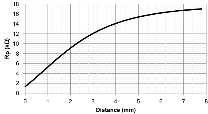
Figure 54. Example R_P vs. Distance with a 14-mm PCB Coil and 2mm Thick Stainless Steel Target
