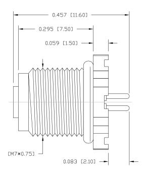
NOTE: MATERIAL HOUSING: PBT UL94V-0, BLACK CONTACT: BRASS NUT: BRASS BRASS SHELL: □-RING: NBR, BLACK FINISH CONTACT: GOLD PLATED OVER 504" NICKEL NUT: NICKEL PLATED NICKEL PLATED SHELL: ELECTRICAL RATED CURRENT: 1A 60V RATED VOLTAGE: 100 MOhms MIN.
