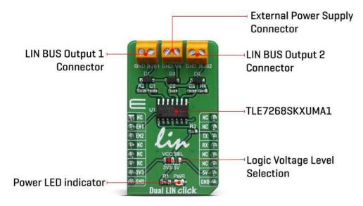
The Dual LIN click communicates with the MCU by using the UART RX and TX signals. RX and TX signals are also routed to the header on the edge of the click board<sup>™</sup> so they can be used independently of the mikroBUS<sup>™</sup> socket. Its most important features are the fact that it is a two separate single-wire LIN transceiver bus for transmission rates up to 20 kbps and it is compliant to ISO 17987-4 and LIN Specification 2.2A.
