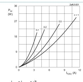
$\begin{array}{l} I_{\text{F(AV)}} = I_{\text{F(RMS)}} \times \sqrt{\delta} \\ V_{\text{o}} = 1.144 \; V; \; R_{\text{s}} = 0.1272 \; \Omega \end{array}$ Fig. 1. Forward power dissipation as a function of average forward current; square waveform; maximum values; per diode
