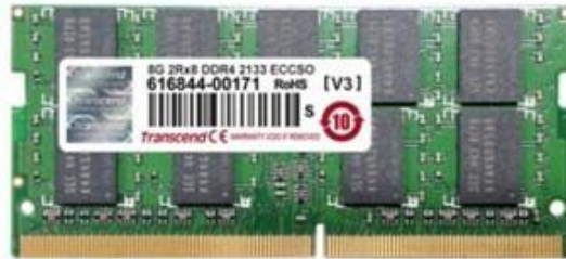
Figure 4-17 Standard DDR4 SO-DIMM with ECC
