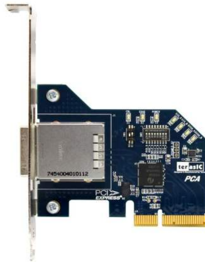
Figure 4-12 PCIe Cabling Adaptor(PCA) card
