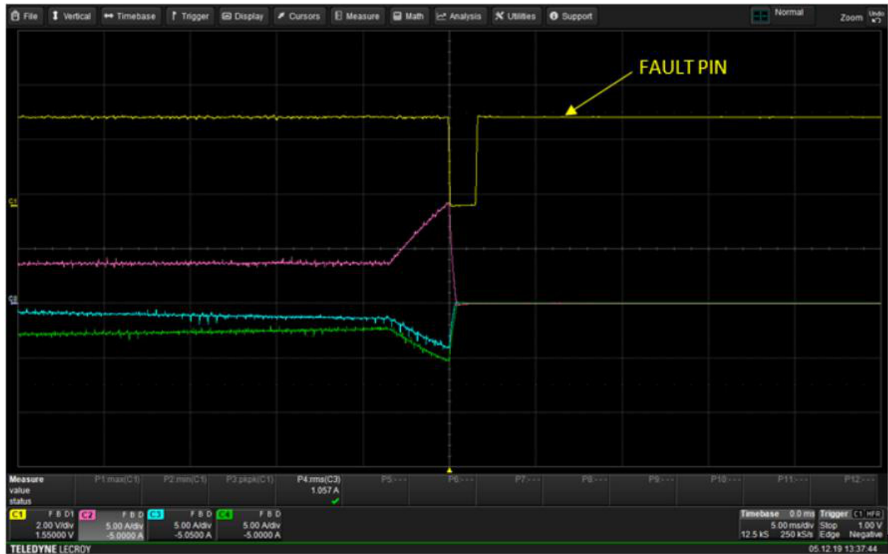
Figure 18. Reaction of Over-current Protection – Detail
