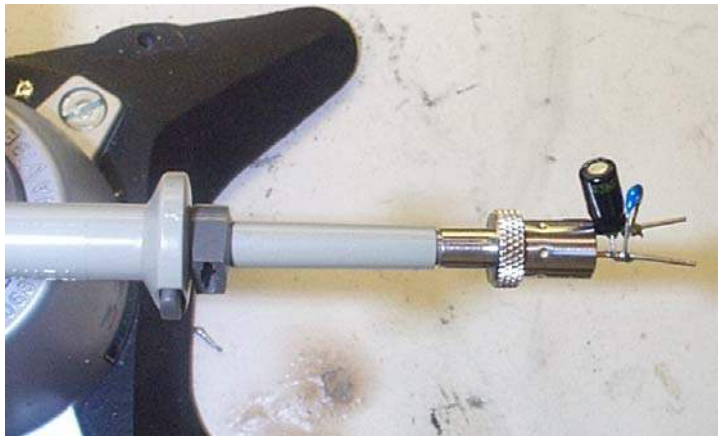
Figure 18 – Oscilloscope Probe with Probe Master 5125BA BNC Adapter. (Modified with wires for probe ground for ripple measurement and two parallel decoupling capacitors added).
