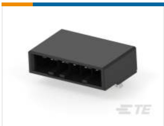
TE Part #1-2347004-5 Header Assembly: Wire-to-Board Connector, Spring Clamp, 5.08 mm pitch, 10A
