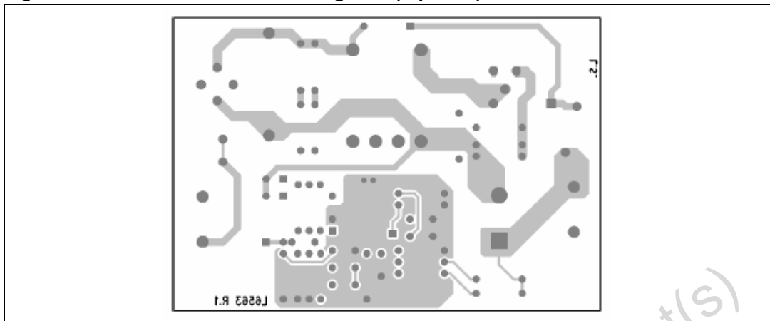
Figure 3. EVAL6563-80W: soldering side (top view)
