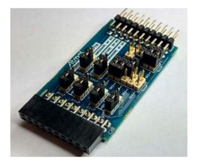
The Atmel® ATBTLC1000-XPRO-ADPT is an adapter board for the ATBTLC1000-XPRO expansion board. It is required for the UART hardware flow control functionality to operate correctly when the ATBTLC1000-XPRO expansion board is connected to certain Atmel Xplained MCU base boards.
