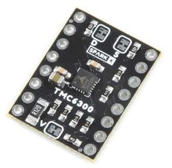
The TMC6300 from Trinamic is a powerful, yet easy to use three phase brushless DC (BLDC) motor driver. Separate high side and low side controls allow for incredible control up to 2A of current. The driver is temperature and short circuit protected with a diagnostic output pin to indicate system issues. With an operating voltage down to 2V, the TMC6300 is suitable for battery powered designs.
