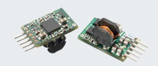
Advanced Energy's Artesyn LDO10C series non-isolated DC-DC converter is designed for cost- and space-sensitive applications. It has a wide 3–13.8 Vdc input range and offers a 0.59–5.1 Vdc adjustable output that accommodates a wide variety of silicon power needs. Capable of delivering up to 10 amps, the converter has a typical efficiency of 94%. A remote enable facility is provided as standard.
