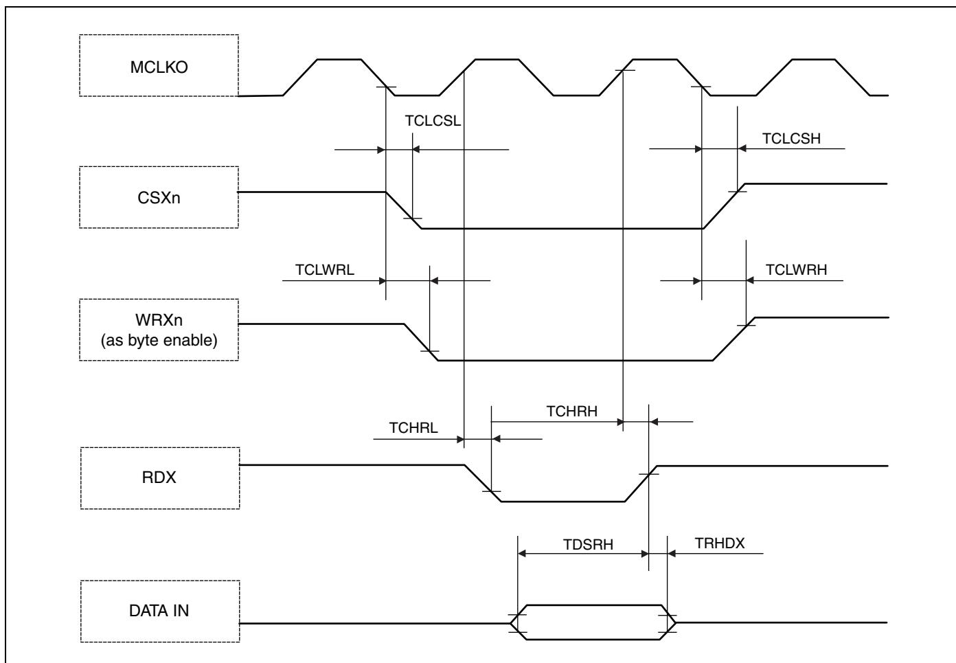
*Synchronous Write Access - Byte Control Type*
