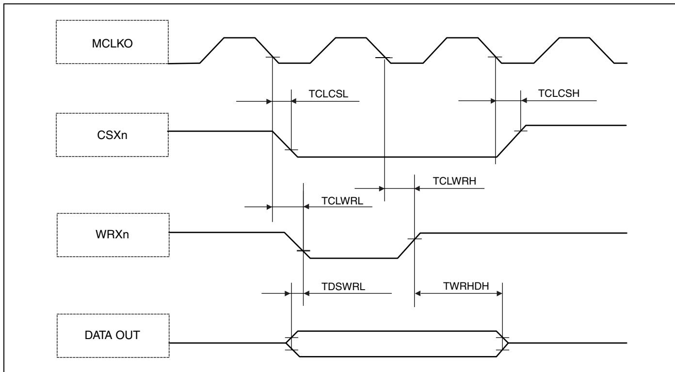
*Asynchronous Write Access - Byte Control Type*
