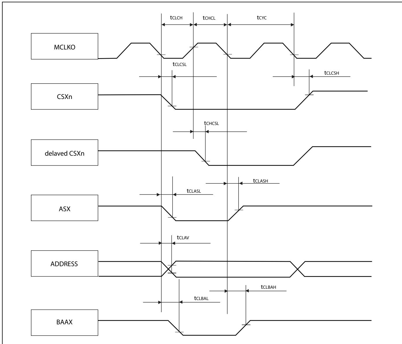
*Synchronous/Asynchronous Read Access With External MclkI Input*
