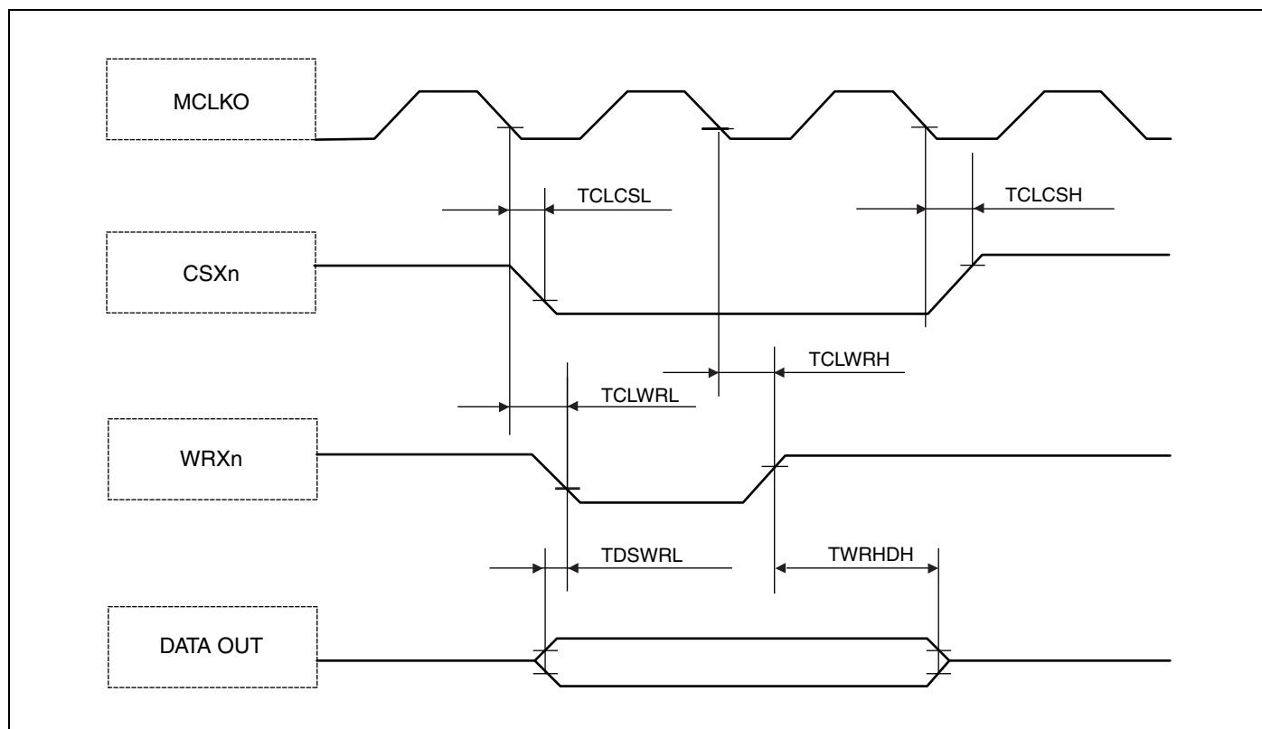
*Asynchronous Write Access - Byte Control Type*
