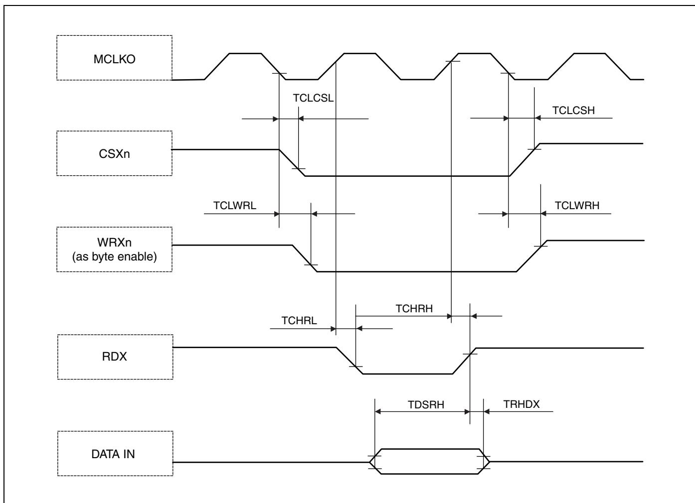
*Synchronous Write Access - Byte Control Type*
