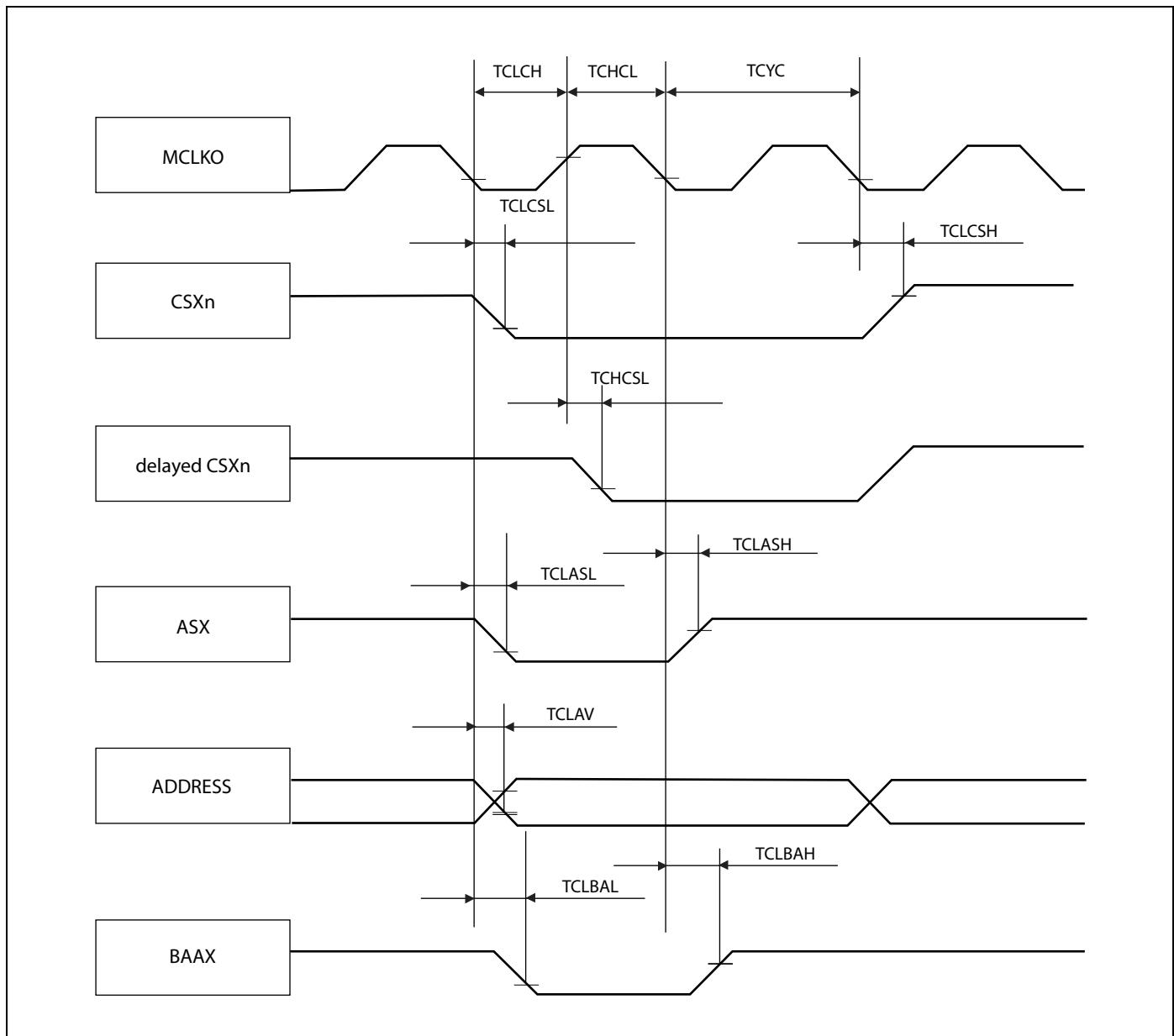
*Synchronous/Asynchronous Read Access With External MclkI Input*
