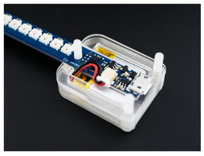
5. Make sure the board is resting flat in piece #5 and add piece #6 to secure it.
