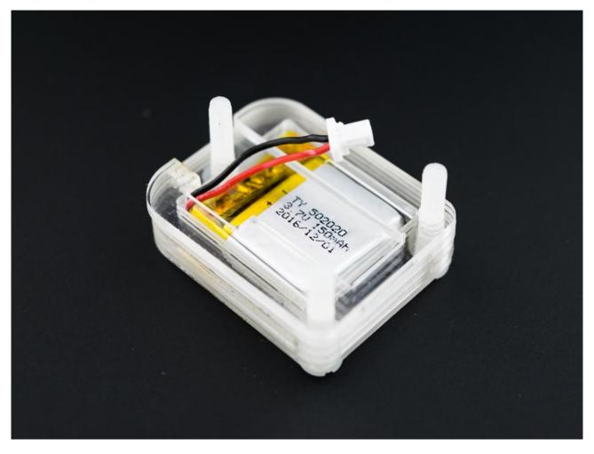
4. Thread the top screw through the hole in the TinySaber board and add it to the stack. Plug the battery in, curving the wires toward the center of the board.
