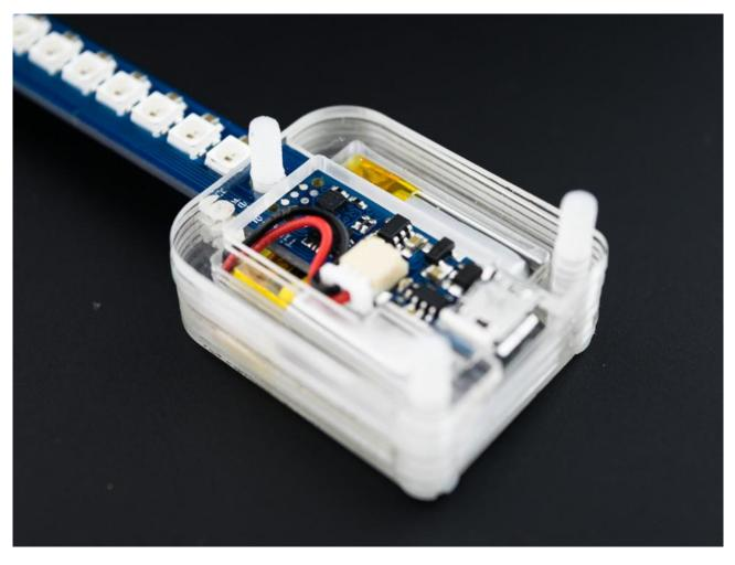
6. Add piece #7, then the top piece. Hand-tighten the nuts onto the screws.
