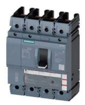
circuit breaker 3VA5 UL frame 250 breaking capacity class C 100kA @ 480V 4-pole, line protection TM230, FTAM, In=150A overload protection Ir=150A fixed short-circuit protection Ii=5...10 x In N conductor unprotected without connection
