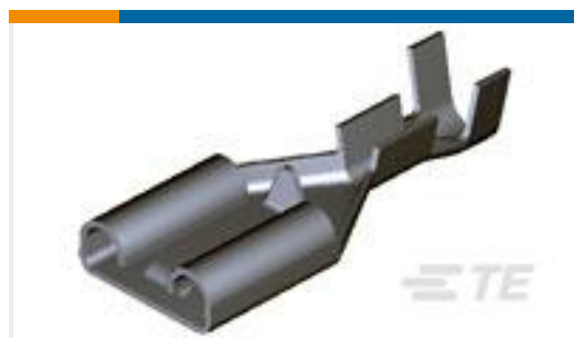
TE Part #63854-2 250 PL MKIII REC. 18-14AWG TPBR
