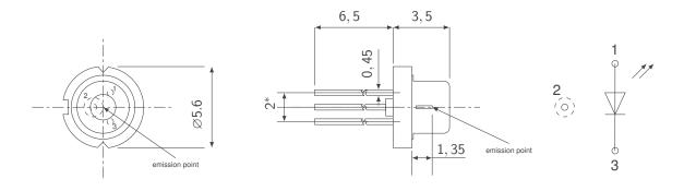
all dimensions in mm. Tolerance  $\pm 0,\, 1$  except given ones \* at the bottom of the LED
